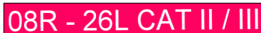
CAT II/III- stop sign (in connection with stop bar and CAT II/III-stop line, at taxi stop CAT II/III)
